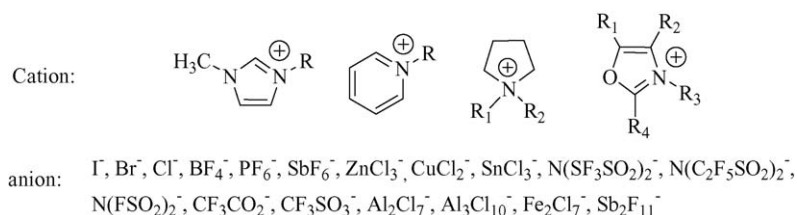
Scheme 1. The constituents of conventionally used ionic liquids.
